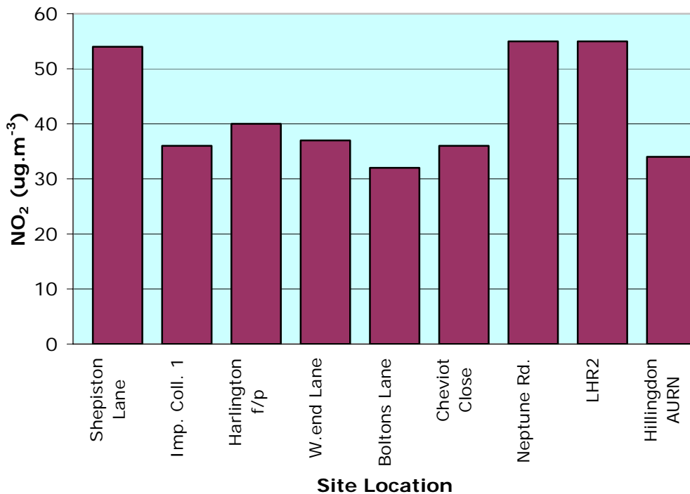
Figure 3: Bias-Adjusted Mean NO 2 Concentrations Using The LHR2 2004-05 Adjustment Factors
