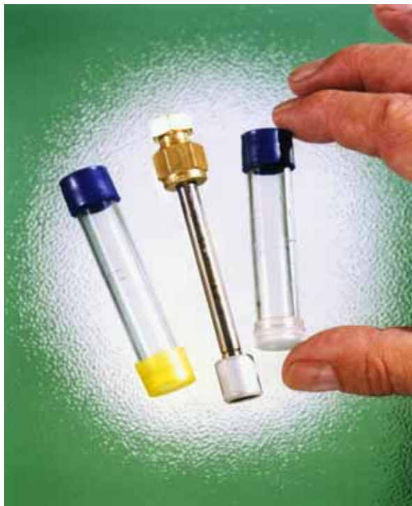
Figure 1: Diffusion Tubes for (left to right) SO 2 , BTX and NO 2
