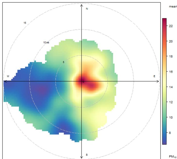
Figure 4.15 (for PM<sub>10</sub>) shows high concentrations occurred under calm conditions very close to the monitoring station (north east and south east). There was also a moderate source shown from approximately 280-290 ° for wind speeds between 5 and 10 ms<sup>-1</sup>. In contrast with the last few years, no relevant PM<sub>10</sub> concentrations seem to excel for higher wind speeds.
