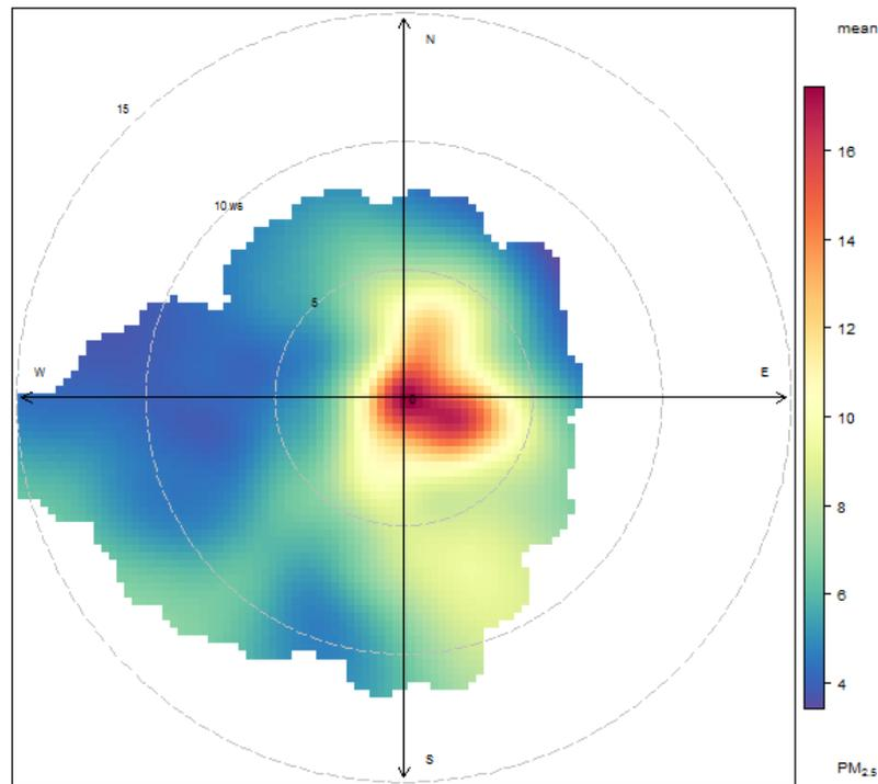
Figure 4.16 shows a similar directional pattern for PM<sub>2.5</sub> to the one seen for PM<sub>10</sub>. At low wind speeds, there appeared to be a build-up close to the monitoring location, suggesting the same sources were involved for both particulate size fractions. The signatures at moderate to high wind speeds were also similar, although PM<sub>2.5</sub> showed a lower contribution than the ones seen for PM<sub>10</sub> (note that the scales vary between Figures 4.15 and 4.16).
