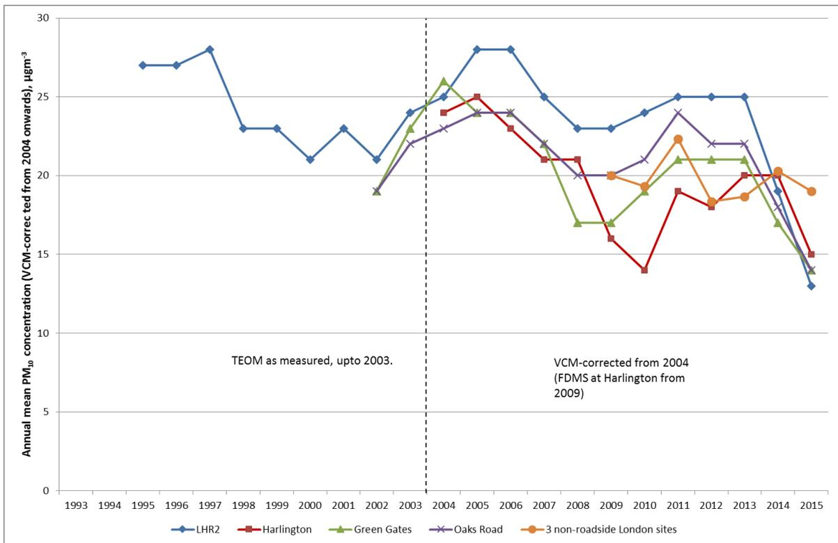
Figure 4.24 shows the annual averages of PM<sub>10</sub> collected for LHR2 since 1995 and for all sites since 2002. Data for 2015 was recorded by a FIDAS instrument, therefore requires no correction factor.
