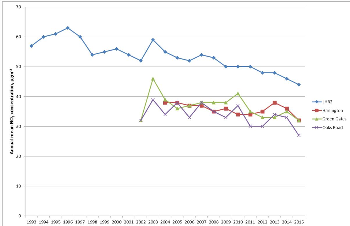
In the case of NO<sub>2</sub> (illustrated in Figure 4.22), there is a stable downward trend at LHR2, although this is less marked than those seen for NO in the previous figures. The annual mean concentrations at Harlington, Green Gates and Oaks Road have fluctuated between 27 µgm<sup>-3</sup> and 39 µgm<sup>-3</sup> apart from two peaks at Green Gates in 2003 and 2010.
